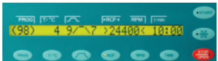
ROTINA 380 R control panel (C control panel)
